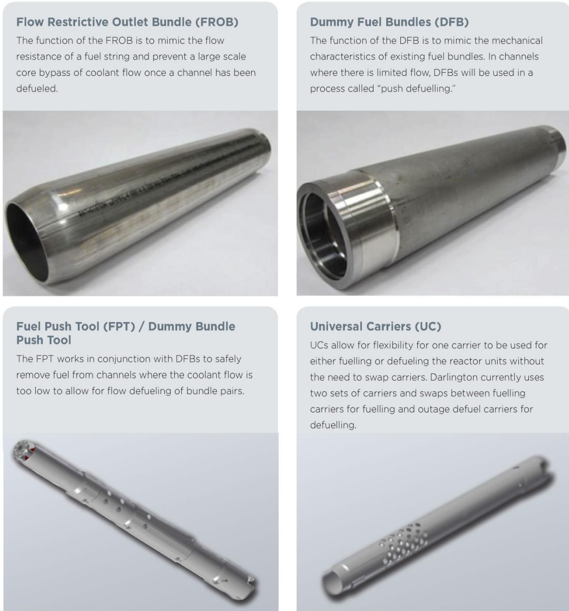
Figure 2 – Universal Carriers and Equipment Required for Defueling
